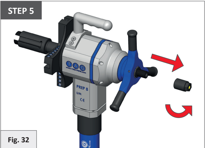
Rotate the lock/unlock nut in anti-clockwise way
