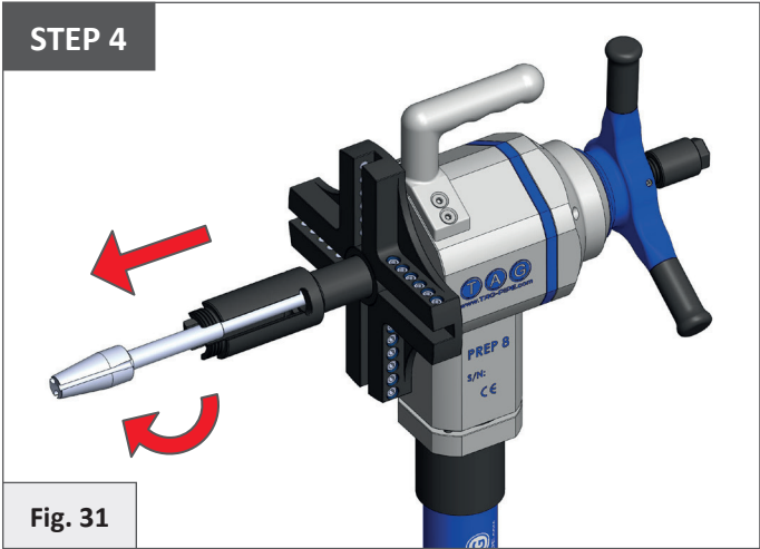
By using long nose pliers rotate clockwise the inside shaft until it comes out
